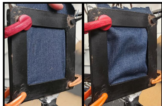
Figure 1. Taut (left) and 1cm loose standoff (right) fabric configurations.
