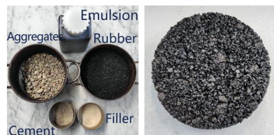
Figure 1. The impact-absorbing pavement material components and the samples.
