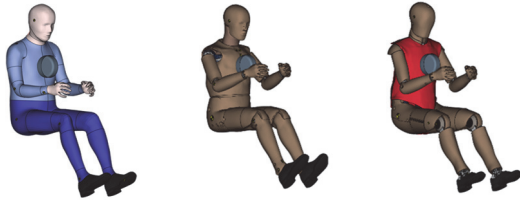
Figure 1: Hub loading for the HBM Connect® 50M, H3-50M and THOR-50M, as shown from left to right for Kroell et al. 1971.
